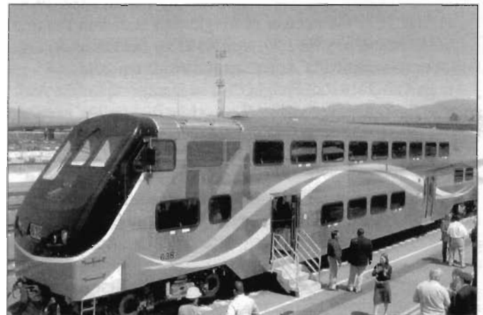
On May 3, Metrolink had two new crushable cars on display at their maintenance yard in Colton. The cab car, shown here, has one end sloping at the upper deck for the driver and the car is crushable at the lower deck: Photo by Andrew Novak
