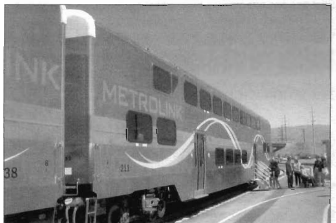
The cab car's second end, shown at left, and both ends of a trailer car, No. 211 at right, are vertical and the lower deck is crushable. Photo by Andrew Novak
