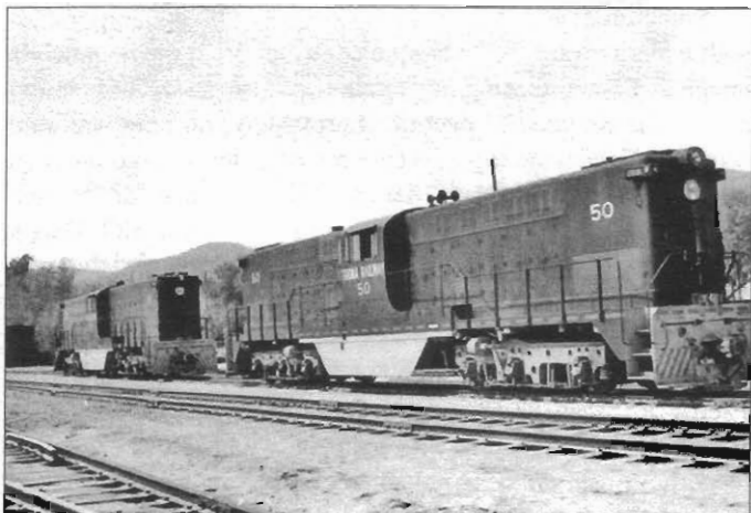
Baldwin 2000 hp center cabs 50 or 51 arrive on the Trona in 1949 and were most likely the power on "Big Red's" Trona picnic train. Photo by Dick Donat
