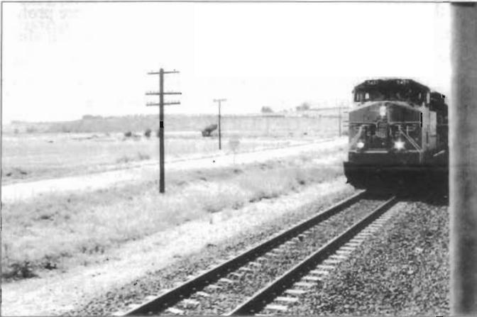
*UP 5437 leads a Southbound General Merchandise Freight at Bena, as seen from Entertainment Car Pony Express. In the distance to the left of the locomotive, are three more locomotives being used in Distributed Power Configuration, which has eliminated the need for manned helpers.*
